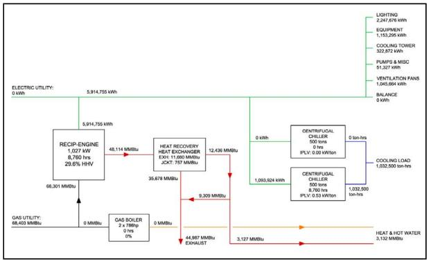
Figure 8-1: CHP System Schematic
