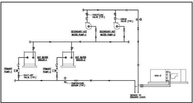
Figure A-3: Hot Water Flow Schematic
