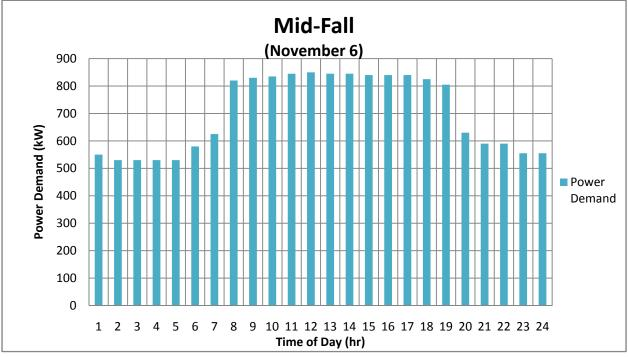
Figure C-1 - The following figures are the electric load profiles for the Pediatric Inpatient Addition for four typical days throughout a given year. The generator for CHP will operate under these conditions year round.
